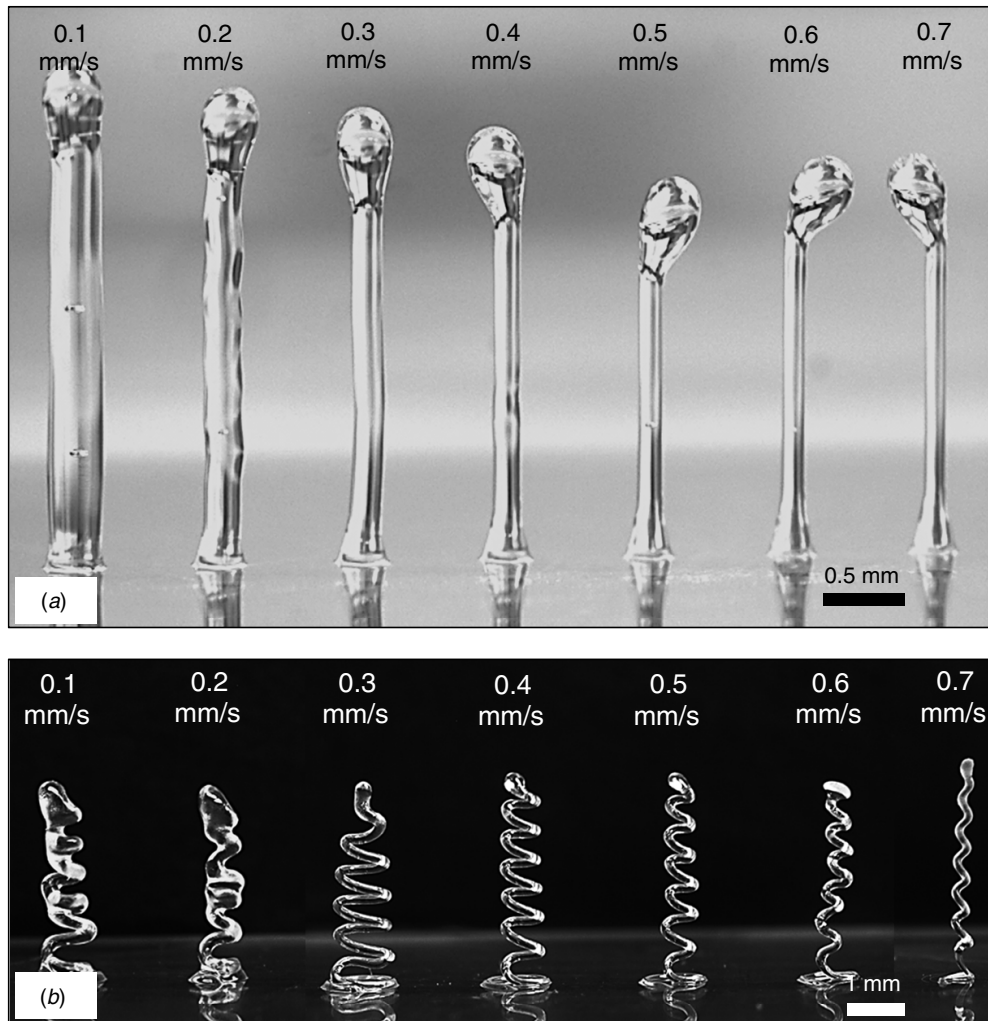
Figure 7. UV-3DP fabrication of (a) vertical filaments and (b) freeform microsprings at different deposition speeds and a constant extrusion pressure of \sim 1 MPa using an extrusion nozzle of 150 \mu\text{m} -internal diameter and the UV-PU resin, NEA 123T.
